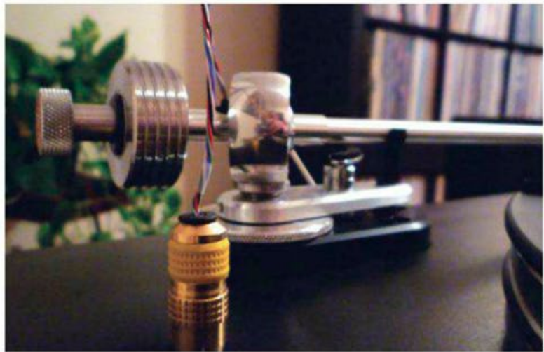
The Traveler's 10"-long, spring-loaded tonearm uses a gimbal bearing.
