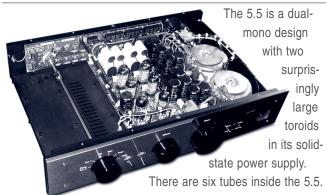
The input stage runs directly to two 12AX7 tubes, which are the first differential gain stage. The two other pairs of tubes are output to the differential buffer stage—one tube for each leg of the signal for the left and right channel so it has a balanced output section.
